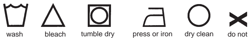
Figure 3. ASTM Symbol System—Basic Symbols
